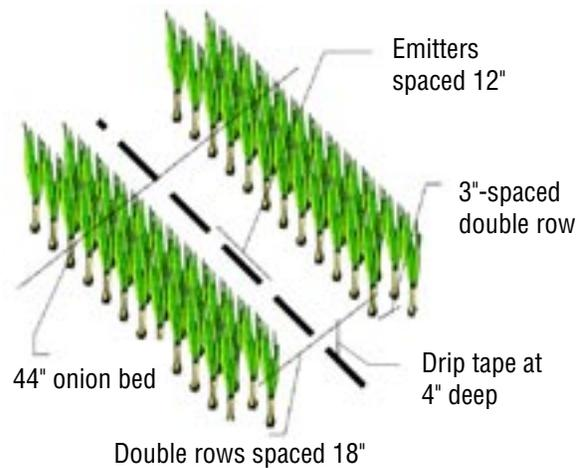
*Figure 1. Typical bed configuration for drip-irrigated onions. On 44-inch beds, two double rows are centered 18 inches apart. Double rows consist of two onion rows spaced 3 inches apart. Drip tapes are installed 3 to 4 inches deep in the bed center. Tape emitters are 12 inches apart.*
