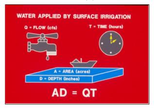
plane. If the faucet is turned on for a specified time (T), the result will be a known depth of water (D) in the container. The same is true of irrigation systems. For example, in rill irrigation, one cubic foot per second of water (Q) set on one acre (A) for one hour (T) will result in a one inch gross
